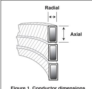
Figure 1. Conductor dimensions are measured in the axial and radial directions of the transformer coil.
