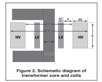
mension) x 7 mm. The LV coil has 2 layers that are separated by a cooling duct, resulting in a "b1" dimension of 12 mm (see Figure 2). The space between the HV and LV windings (dimension "a") is 20 mm.
